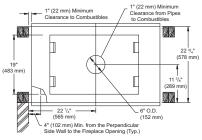
Figure 3 - Clearances from Top View
